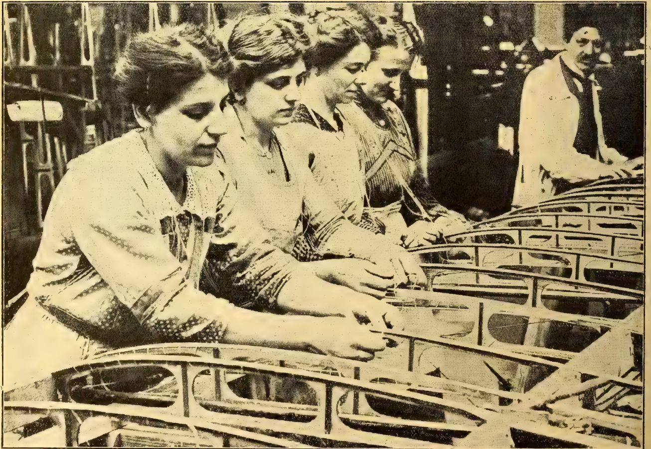
GERMAN AEROPLANE PRODUCTION.—A photograph of the wing assembling work in the Albatros Factory. Fabric strips are being strung onto the ribs to make a lining between the rib and the doped fabric on top. It may be noticed that the workers do not show any noticeable signs of starvation, despite the stories of which we hear so much.
